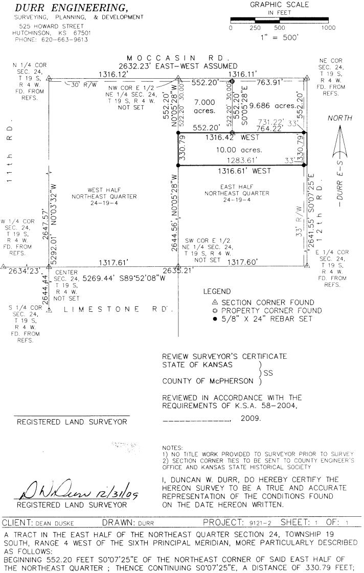
THE NORTHEAST QUARTER; THENCE CONTINUING S0°07'25"E, A DISTANCE OF 330.79 FEET; THENCE WEST, A DISTANCE OF 1316.61 FEET TO THE WEST LINE SAID EAST HALF; THENCE NO 05'28"W, A DISTANCE OF 330.79 FEET; THENCE EAST, A DISTANCE OF 1316.42 FEET TO THE POINT OF BEGINNING; TRACT CONTAINS 10.00 ACRES, EXCEPT THE EAST 33 FEET FOR ROAD RIGHT OF WAY AND ANY OTHER EASEMENTS OF RECORD: ALL IN McPHERSON COUNTY, KANSAS. TWP: 19 S DATE: 12/31/2009
