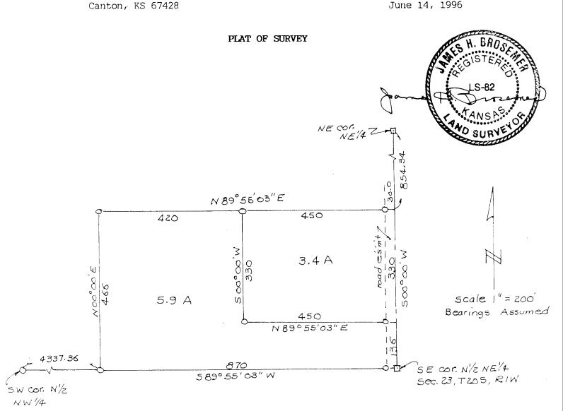
Legend:  $0 = \frac{1}{2}$  rebar with IO cap (set)  $\Pi = \frac{5}{8}$  rebar (found)
