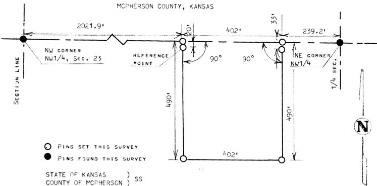
I, Melvin Ferguson, Professional Engineer of the state of Kansas do Hereby Gertify that under my supervision a survey was made of a tract of land in the NW1/4, Section 23, T19S, R2W of the 6th P.M. and described as follows; Commencing at the NW corner of the NW1/4, Section 23, T19S, R2W; thence East on Section Line 2021.9 feet for place of Beginning; thence continuing East
