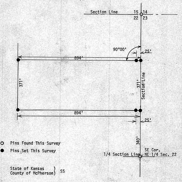
I, F. R. Rankin, County Engineer of McPherson County, Kansas, do hereby certify that under my supervision a survey was made in the NE 1/4 Section 22, T17S, R4W of the 6th P.M. and described as follows:
