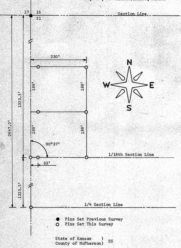
I, F. R. Rankin, County Engineer of McPherson, Kansas, do hereby certify that under my supervision a survey was made of a tract of land in the NW1/4, NW1/4 of Section 21, T21S, R4W of the 6th P.M. and described as follows:
