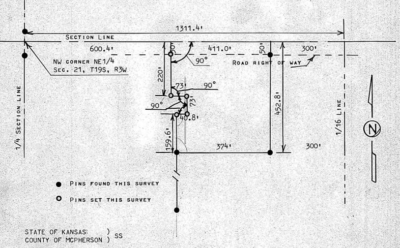
1, Melvin Ferguson, Professional Engineer of the state of Kansas do Hereby certify that under my supervision a survey was made in the NW1/4,NE1/4, Section 21, T195, R3W of the 6th P.M. and described as follows;
