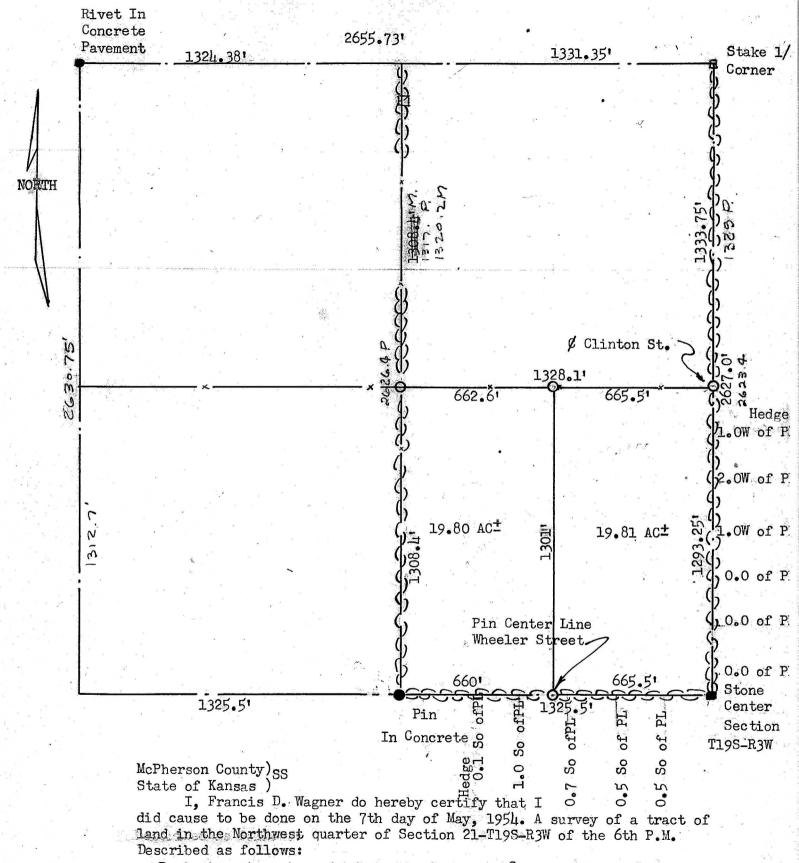
Beginning at a stone which is the Center of Section 21-T19S-R3W of the 6th P. M; thence 1293.25' feet North along the quarter section line between the NE & NW quarters; thence 665.5' feet West; thence 1301' feet South to the quarter section line between the NW & SW quarter; thence 665.5' East to place of beginning tract of land contains 19.81 Acres. ±
