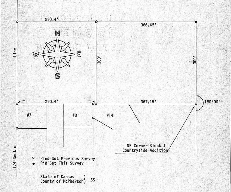
I, F. R. Rankin, County Engineer of McPherson, Kansas, do hereby certify that under my supervision a survey was made in the NW 1/4, SW 1/4, NE 1/4 Section 21, T19S, R3W of the 6th P.M. and described as follows:
