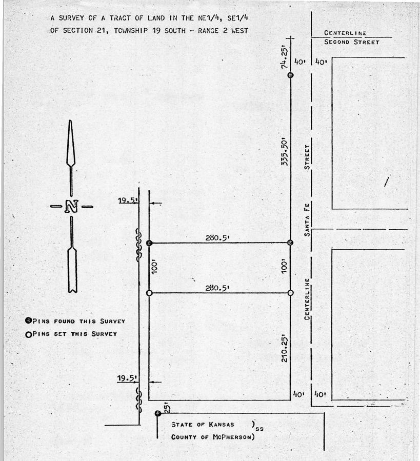
1, F. R. RANKIN, COUNTY ENGINEER OF MCPHERSON COUNTY, KANSAS, DO HEREBY CERTIFY THAT UNDER MY SUPERVISION A SURVEY WAS MADE OF A TRACT OF LAND IN THE NE1/4, SE1/4 OF SECTION 21, T19S - R2W OF THE 6TH P. M. AND DESCRIBED AS FOLLOWS:
