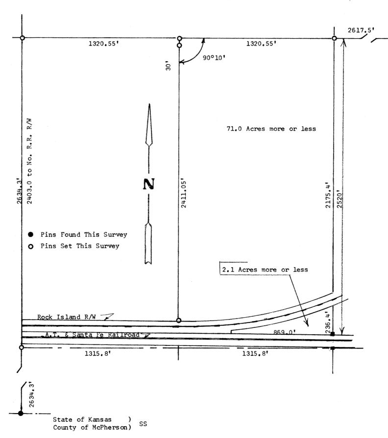
I, F. R. Rankin, County Engineer of McPherson County, Kansas, do hereby certify that under my supervision a survey was made of the El/2, NW 1/4, of Section 21, T19S, R1W of the 6th P.M. That land lying North of the Atchison, Topeka and Santa Fe Railroad and except that part used for Chicago Rock Island and Pacific Railroad. Said tract of land contains 73.1 acres more or less and that the accompanying plat is a true exhibit of said survey.
