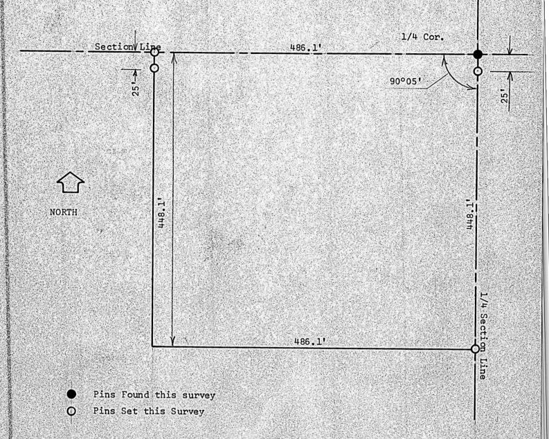
I, F. R. Rankin, County Engineer of McPherson County, Kansas, do hereby certify that under my supervision a survey was made of a tract of land in the NW 1/4 of Section 20, T19S, R4W of the 6th P.M. and is described as follows:
