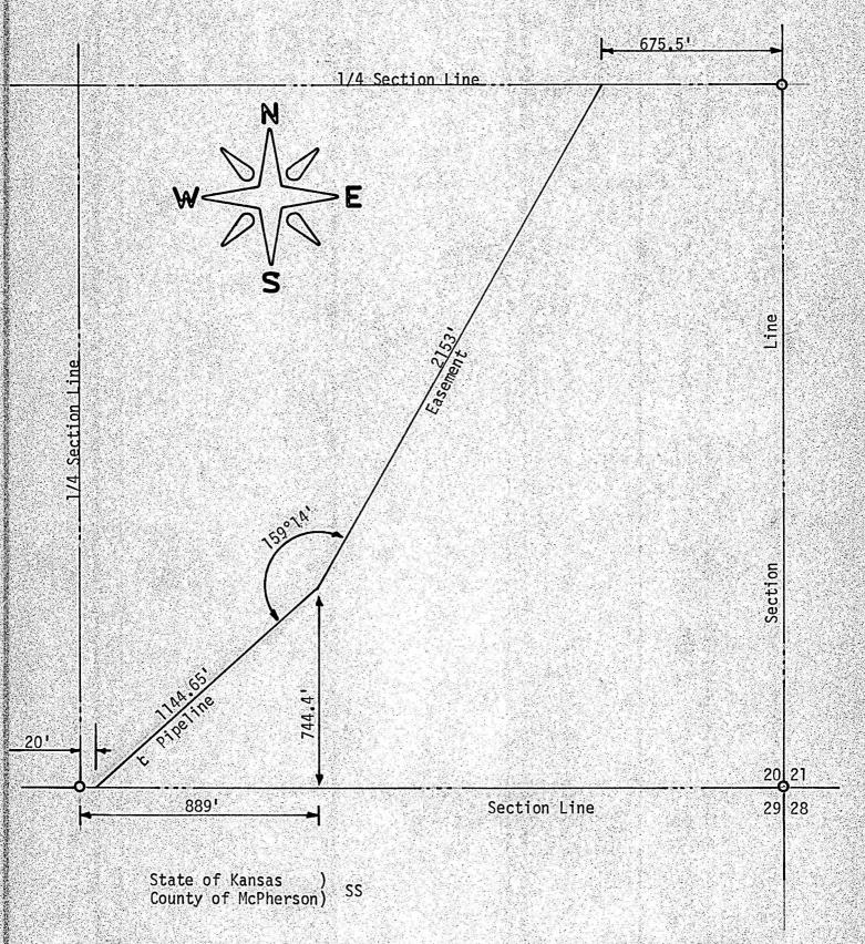
I, F. R. Rankin, County Engineer of McPherson County, do hereby certify that under my supervision a survey was made in the SE 1/4 Section 20, T19S, R4W of the 6th P.M. to determine a pipeline easement and described as follows:
