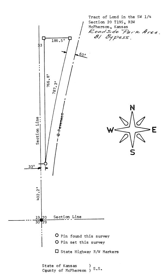
I, F.R. Rankin, County Engineer of McPherson Kansas, do hereby certify that under My supervision a survey was made in the SW 1/4 Section 20 T19S R3W of the 6th. P.M. and described as follows:
