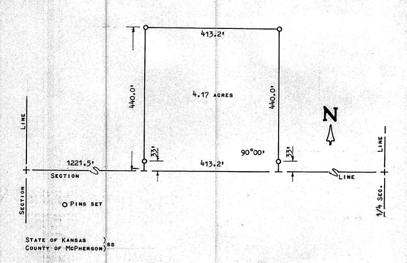
THAT UNDER MY SUPERVISION A SURVEY WAS MADE OF A TRACT OF LAND IN THE SW1/4 OF SECTION 19, T205 - R5W OF THE 6TH P.M. AND DESCRIBED AS FOLLOWS:
