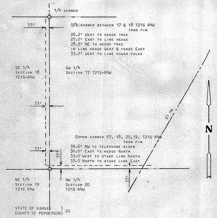
I, Francis Rankin, Professional Engineer of the state of Kansas do Herby Certify that under my supervision a survey was made to determine the Right-of-Way, (stake at 33 feet from section lines) between the SE 1/4 of Section 18 and the SW 1/4 Section 17 T21S R4W, and between the SW 1/4 section 17 and the NW 1/4 Section 20, T21S R4W, and that the accompanying PLAT IS a True exhibit of Said Survey as far as it is known to me.
