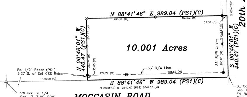
Sec. 17, T19S, R2W Fd. 5/8" Rebar (PS2) Origin Unknown
