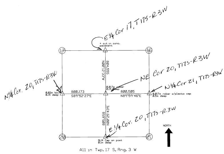
I hereby certify this drawing to be a true and correct representation of a survey conducted by the Kansas Department of Transportation for project 81B-59-K7981-01 dated Oct. 2000, in McPherson County, Kansas
