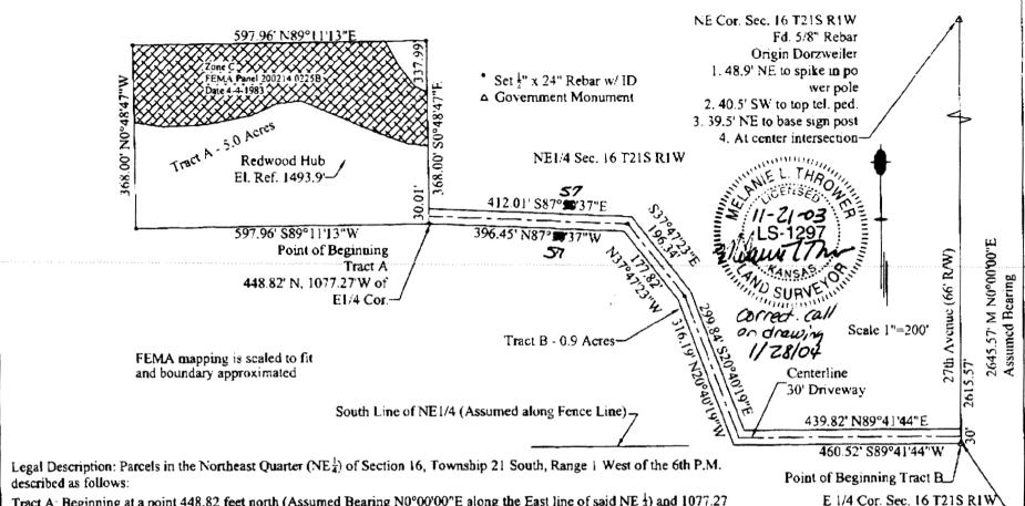
Tract A: Beginning at a point 448.82 feet north (Assumed Bearing N0°00'00"E along the East line of said NE \( \frac{1}{4} \)) and 1077.27 feet west of the Southeast Corner of said NE \( \frac{1}{4} \) Section 16; thence S89°11'13"W a distance of 597.96 feet; thence N0°48'47"W a distance of 368.00 feet; thence N89°11'13"E a distance of 597.96 feet; thence S0°48'47"E a distance of 368.00 feet to the point of beginning containing 5.0 acres more or less; and
