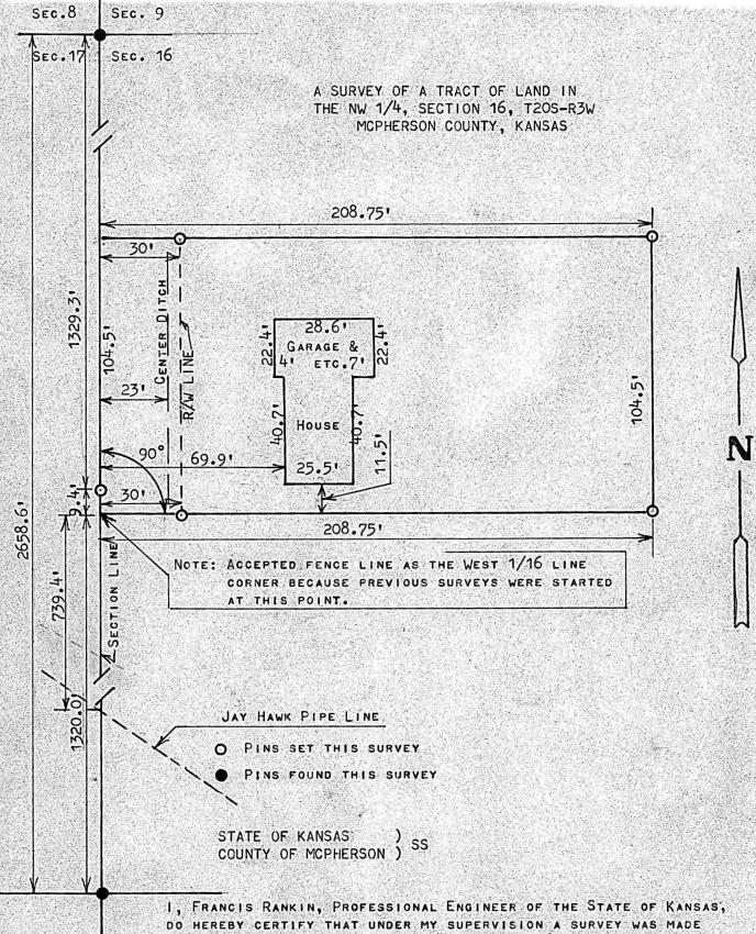
T, FRANCIS KANKIN, PROFESSIONAL ENGINEER OF THE STATE OF KANSAS, DO HEREBY CERTIFY THAT UNDER MY SUPERVISION A SURVEY WAS MADE OF A TRACT OF LAND IN THE NW 1/4, SECTION 16, T20S R3W OF THE 6TH P.M. AND DESCRIBED AS FOLLOWS:
