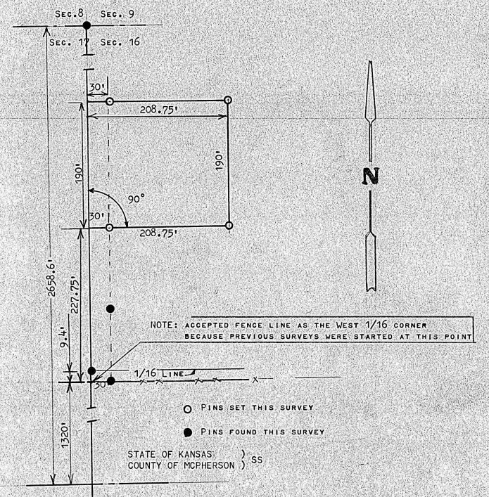
I, FRANCIS RANKIN, PROFESSIONAL ENGINEER OF THE STATE OF KANSAS, DO HEREBY CERTIFY THAT UNDER MY SUPERVISION A SURVEY WAS MADE OF A TRACT OF LAND IN THE NW1/4, SECTION 16, T20S R3W OF THE 6TH. P.M. AND DESCRIBED AS FOLLOWS;
