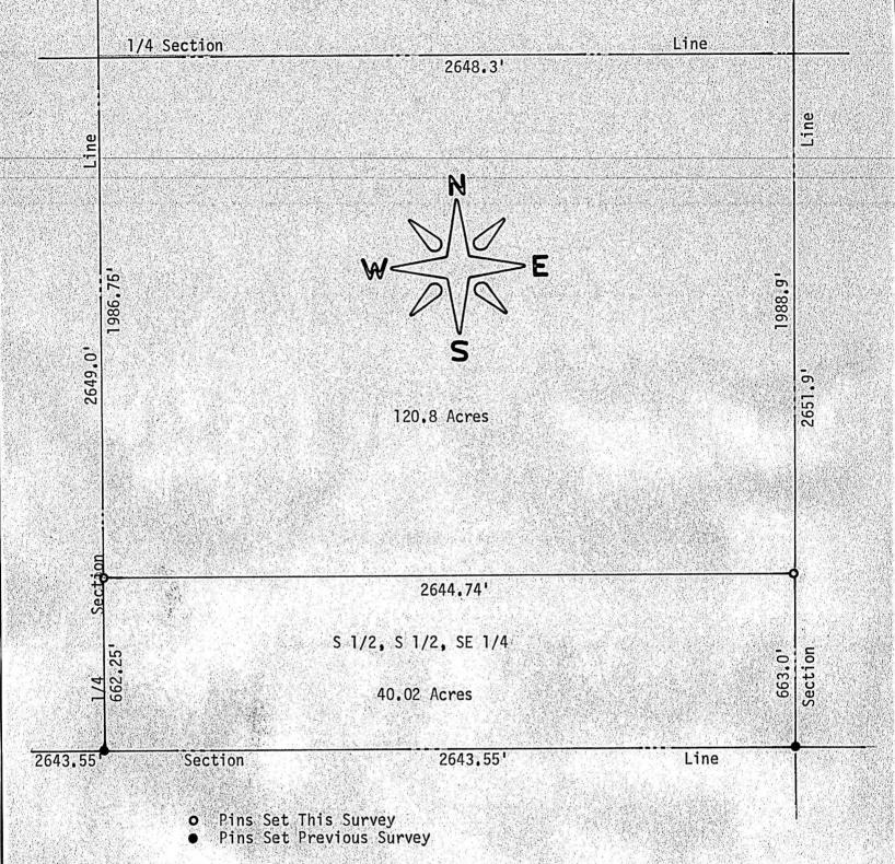
I, F. R. Rankin, County Engineer of McPherson, Kansas, do hereby certify that under my supervision a survey was made of the S1/2, S1/2, SE1/4 Section 16, T18S, R5W of the 6th P.M. and the above plat is a true exhibit of said survey as far as it is Known to me.
