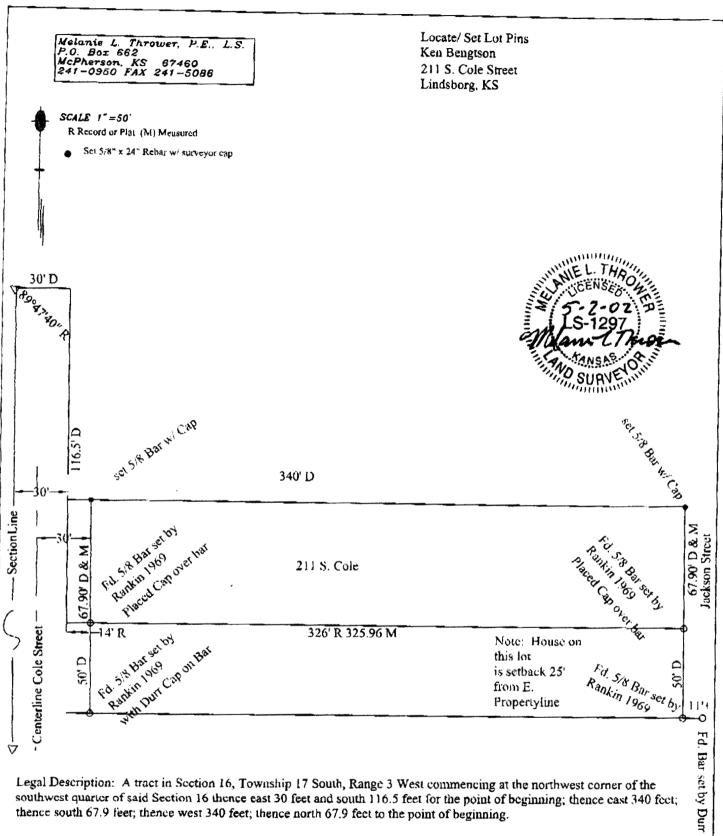
Right of Way Cole Street is 30' from centerline of street according to KDOT road plans dated 1937 and 1993.
