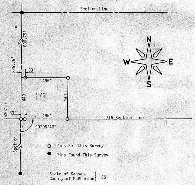
I, F. R. Rankin, County Engineer of McPherson County, Kansas, do hereby certify that under my supervision a survey was made in the N 1/2 of the NW 1/4 of Section 15, T21S, R5W of the 6th P.M. and described as follows:
