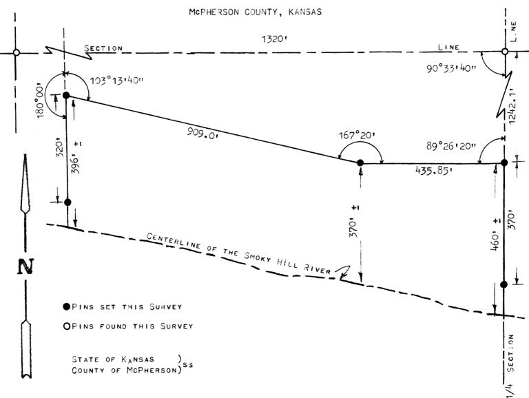
1, MELVIN FERGUSON, REGISTERED LAND SURVEYOR OF THE STATE OF KANSAS, DO HEREBY CERTIFY THAT UNDER MY SUPERVISION A SURVEY WAS MADE OF A TRACT of Land in the NW1/4 of Section 15, T175 - R5W of the 6th P.M. and desc-RIBED AS FOLLOWS:
