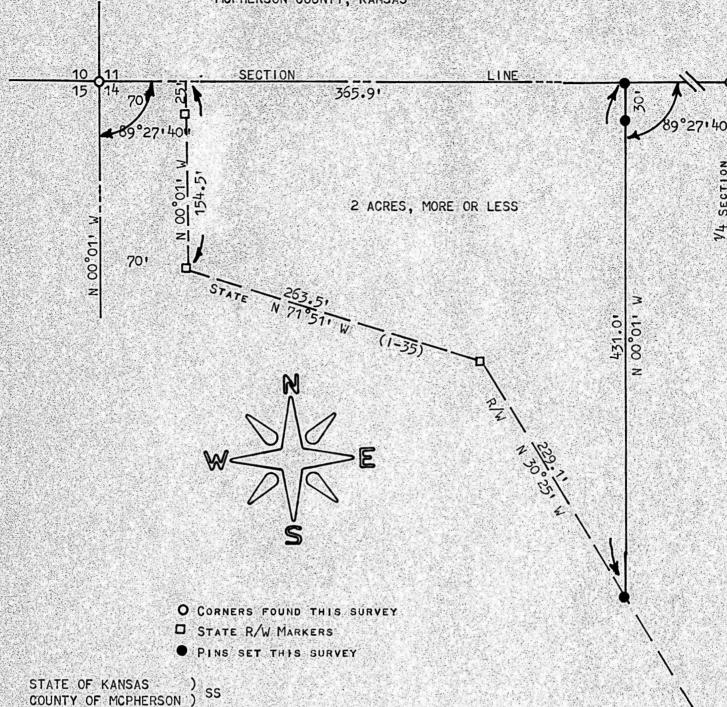
I, F. R. Rankin, County Engineer of McPherson County, Kansas, do hereby certify that under my supervision a survey was made of a tract of land in the NW  $^{94}$ , Section 14, T21S, R2W of the 6th P.M., and described as follows:
