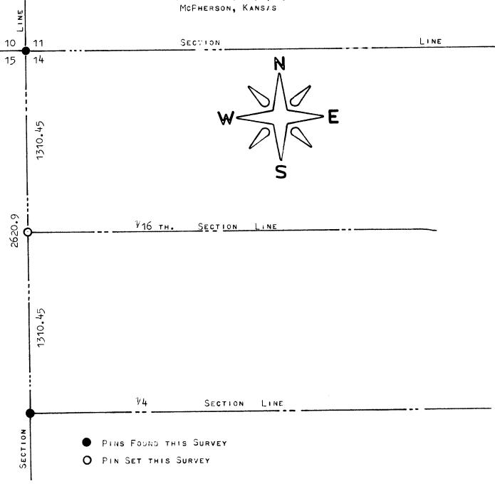
I, F. R. Rankin, County Engineer of McPherson, Kansas, do hereby certify that under my supervision a survey was made in the NW  $^{14}$ 4 Section 14, T19S, R3W, of the 6 P. M. to determine the West  $^{17}$ 16th. corner of the NW  $^{14}$ 4 and the above plat is a true exhibit of said survey as far as it is known to Me.
