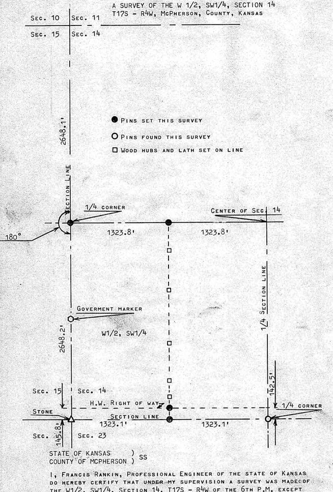
I, FRANCIS RANKIN, PROFESSIONAL ENGINEER OF THE STATE OF KANSAS DO HEREBY CERTIFY THAT UNDER MY SUPERVISION A SURVEY WAS MADECOFTHE W1/2, SW1/4, SECTION 14, T17S - R4W OF THE 6TH P.M. EXCEPT THAT LAND USED FOR HIGHWAY RIGHT OF WAY, AND THAT THE ABOVE PLAT IS A TRUE EXHIBIT OF SAID SURVEY AS FAR AS IT IS KNOWN TO ME.
