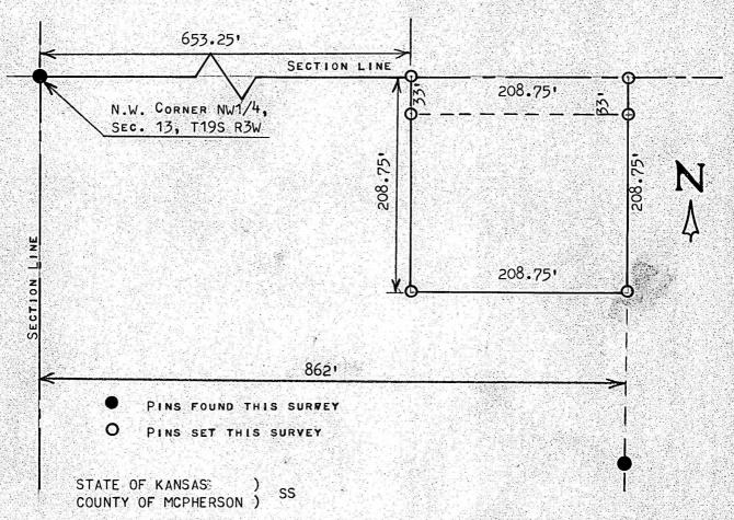
I, Melvin Ferguson, Professional Engineer of the State of Kansas, do hereby certify that under my supervision a survey was made of a tract of Land in the NW1/4, Section 13, T19S, R3W of the 6th. P.M. and described as follows;
