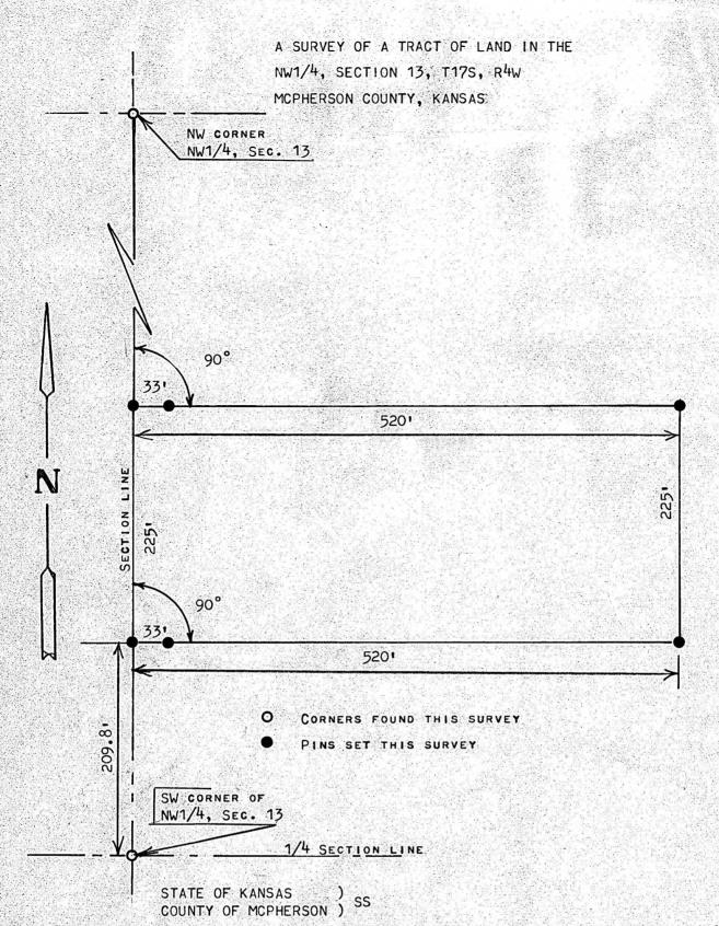
I, Melvin Ferguson, Professional Engineer of the state of Kansas do Hereby certify that under my supervision a survey was made of a Tract of Land in the NW1/4, Section 13, T17S, R4W of the 6th P.M. and described as follows:
