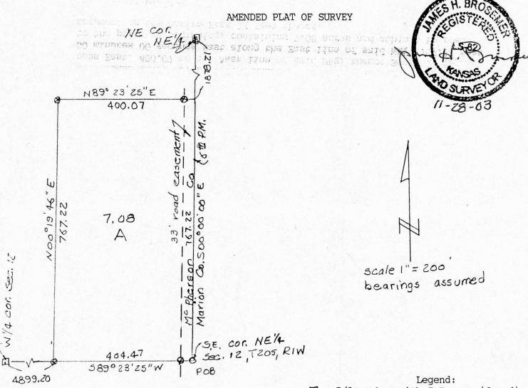
$\Box$  = 5/8" rebar with I.D. cap (found)  $\bigcirc$  = 1/2" rebar (found)
