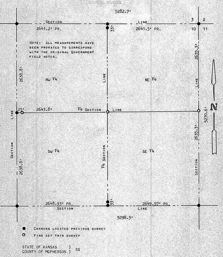
I, F. R. Rankin, County Engineer of McPherson County, Kansas, do hereby certify that under my supervision a survey was made of Section 10, T19S-R4W of the 6th P.M. to establish the  $^{17}4$  Section line between the NW  $^{17}4$  and the SW  $^{17}4$ , Section 10, T19S-R4W, and the above plat is a true exhibit of said survey as far as it is known to me.
