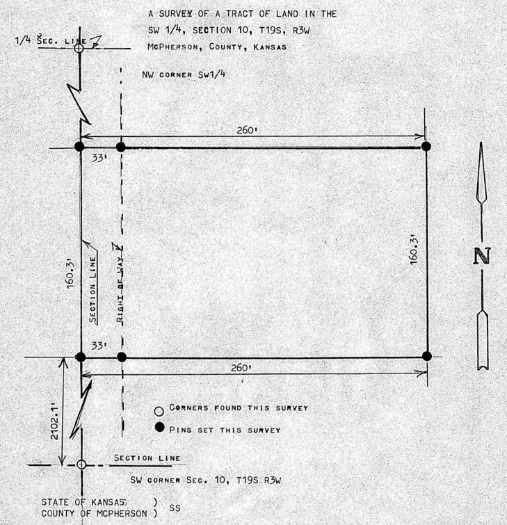
I, Melvin Ferguson, Professional Engineer of the state of Kansas do Hereby CERTIFY THAT UNDER MY SUPERVISION A SURVEY WAS MADE OF A TRACT OF LAND IN THE SW1/4, Section 10, T19S, R3W of the 6th P.M. and described as follows;
