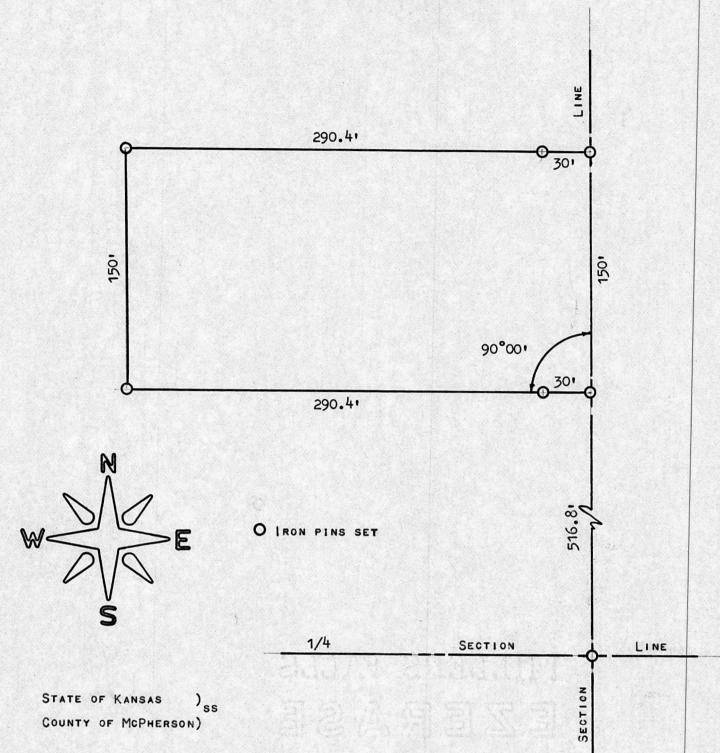
I, F. R. RANKIN, COUNTY ENGINEER OF MCPHERSON CO., KANSAS, DO HEREBY CERTIFY THAT UNDER MY SUPERVISION A SURVEY WAS MADE OF A TRACT OF LAND IN THE NE1/4 OF SECTION 10, T19S - R2W OF THE 6TH P.M. AND DESCRIBED AS FOLLOWS:
