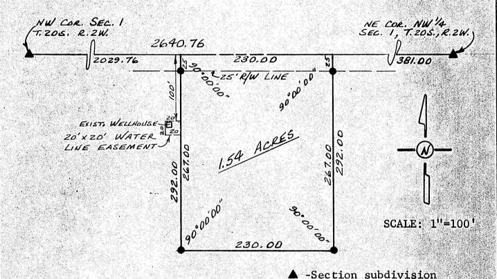
Note: The NE and NW corners of the corn NW½ of Section 1, T20S, R2W of the -5/8" x 6th P.M. were reset by prorating the distances between the NE corner of said Section 1 and the NW corner of the NE½ of Section 3, T20S, R2W of the 6th P.M. Total distance measured was 13,203.79 ft.
